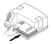
Place the book in the Model 955 as illustrated adjacent. Make sure that the light beam from the optical sensor is not interrupted. The lamp in the "verify" button lights up, indicating that the security strip is sensitive.
