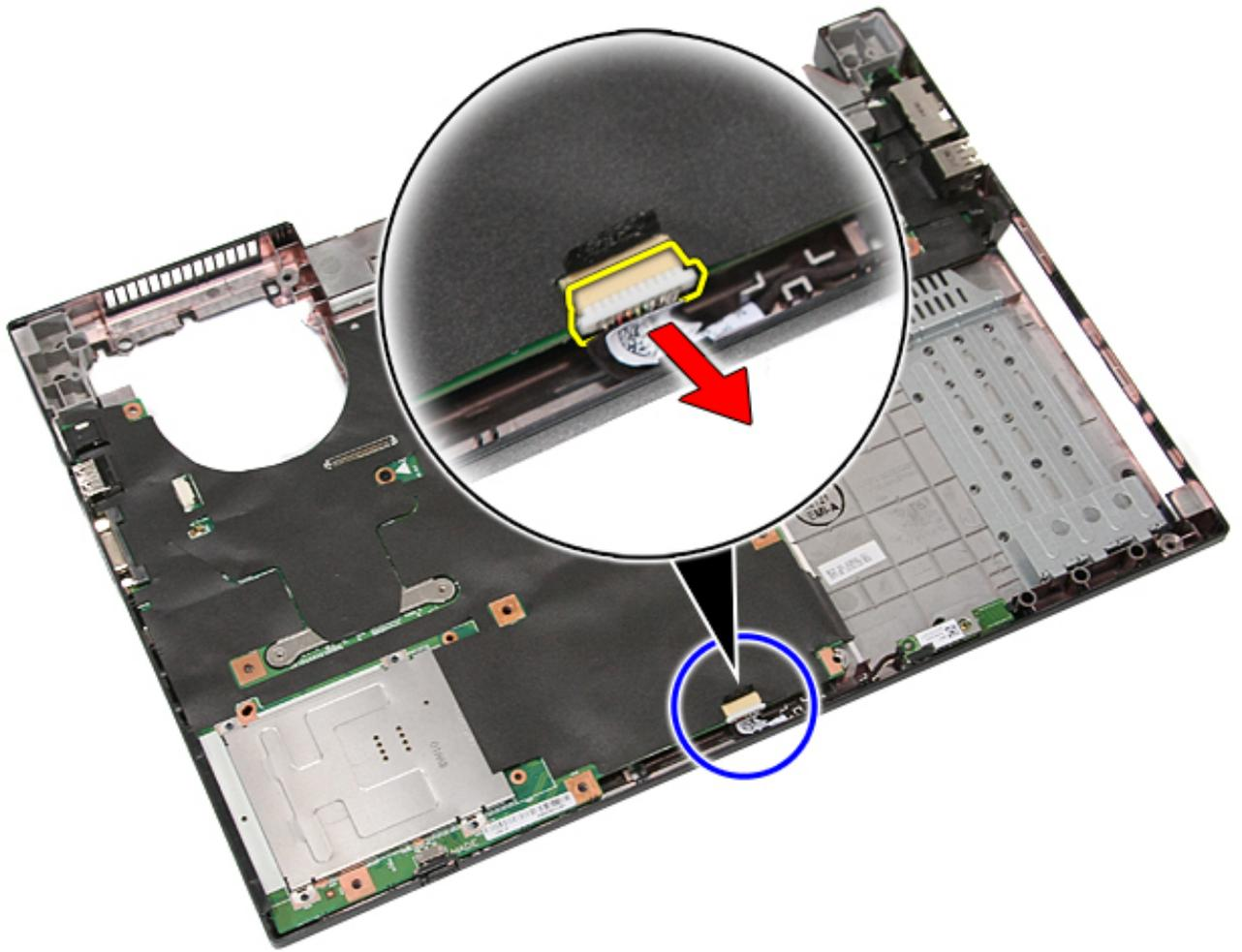
11. Release the Bluetooth board from the latches and remove it.
