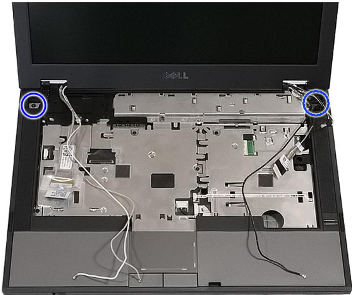
14. Lift up the display assembly from the computer and remove.
