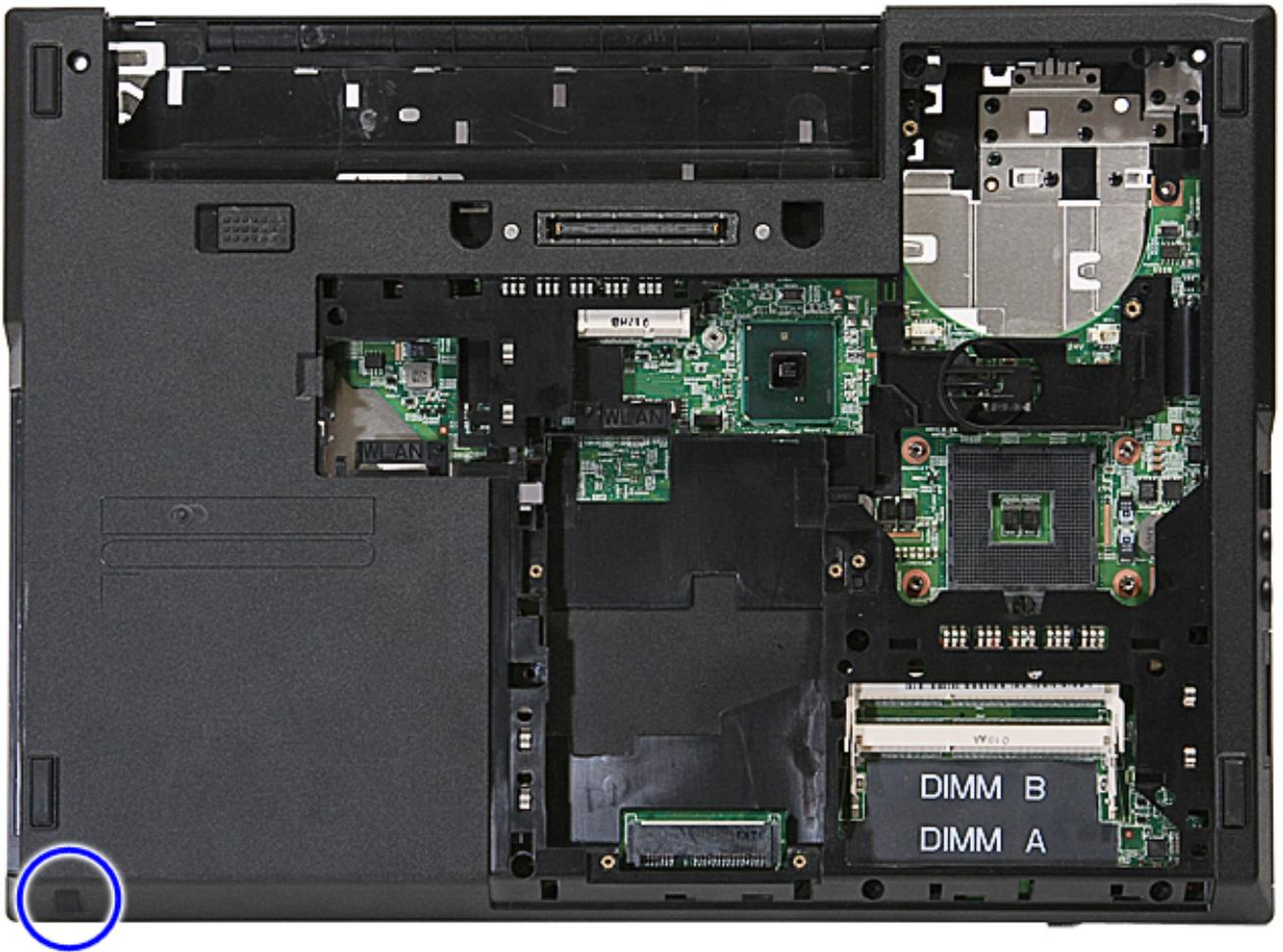
12. Remove the screws securing the palm rest to the computer.
