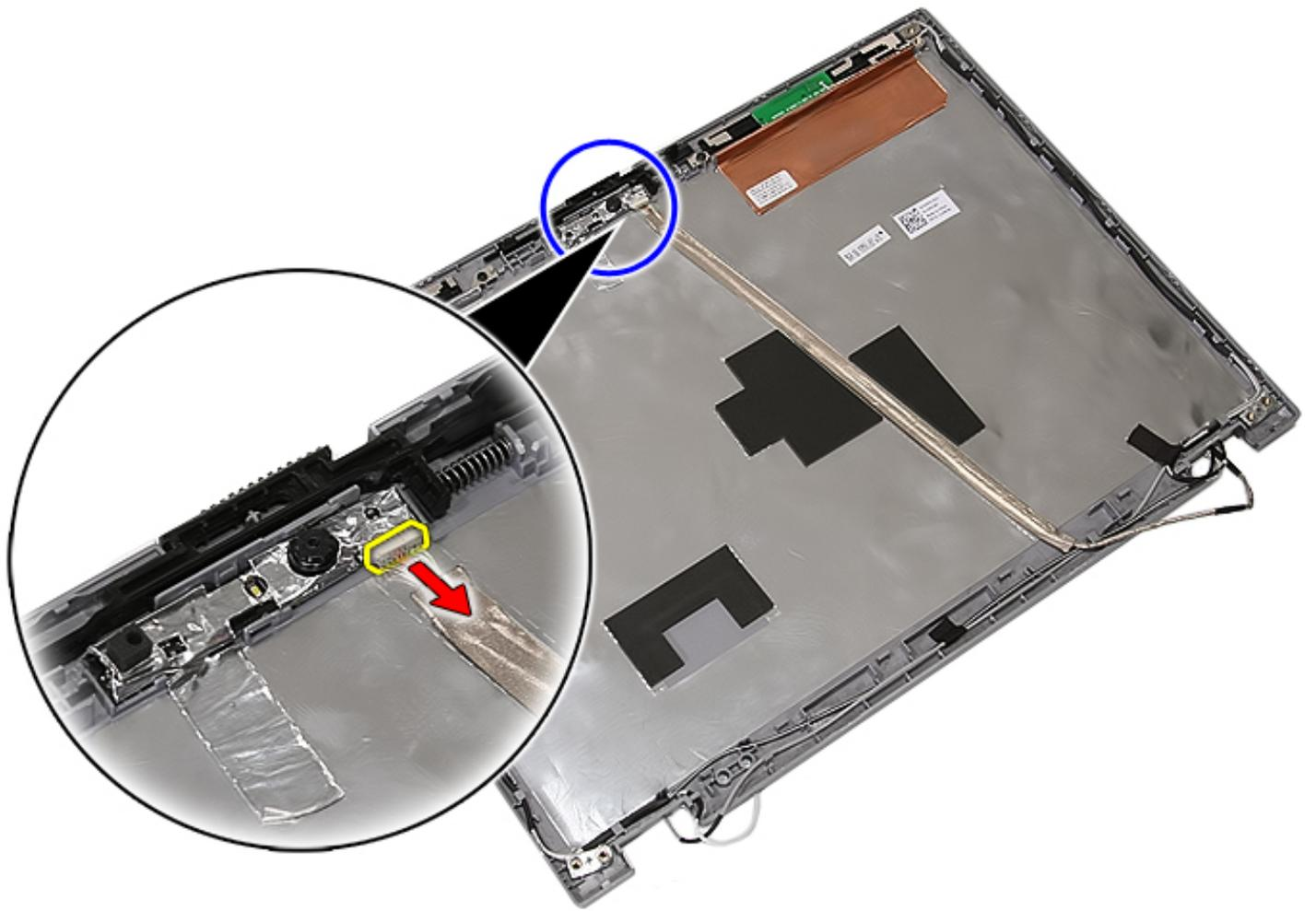
11. Lift up the display camera and remove.
