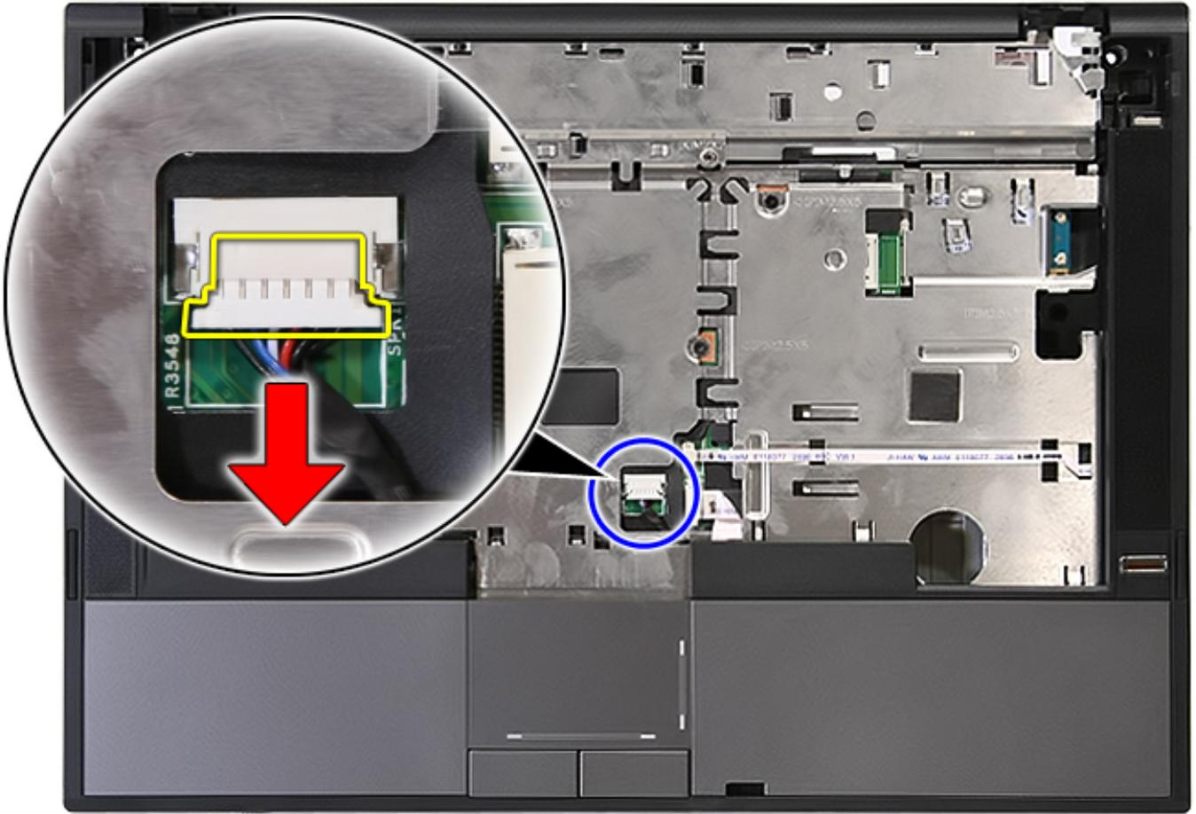
14. Release the latch securing the fingerprint reader data cable.
