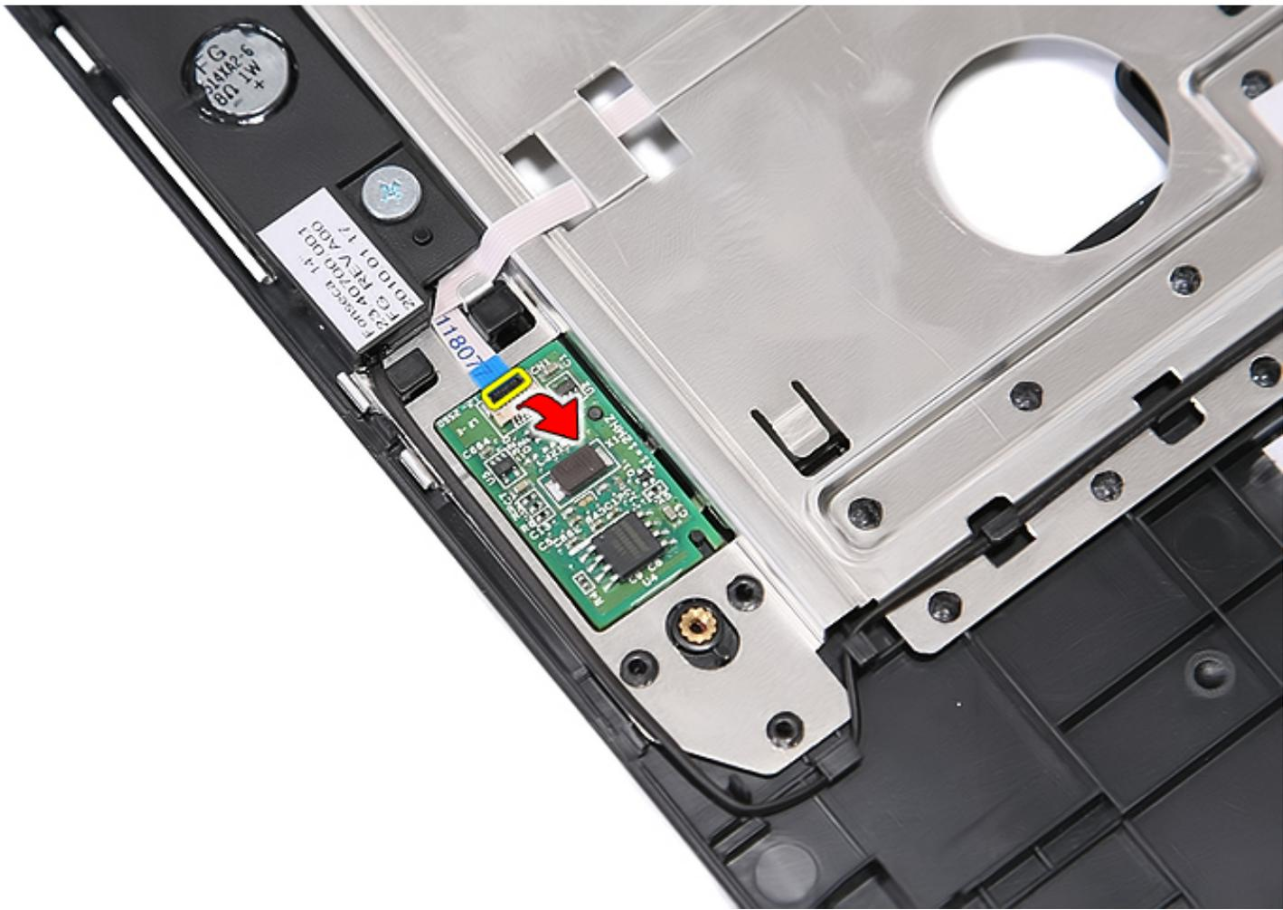
13. Disconnect the fingerprint reader data cable.
