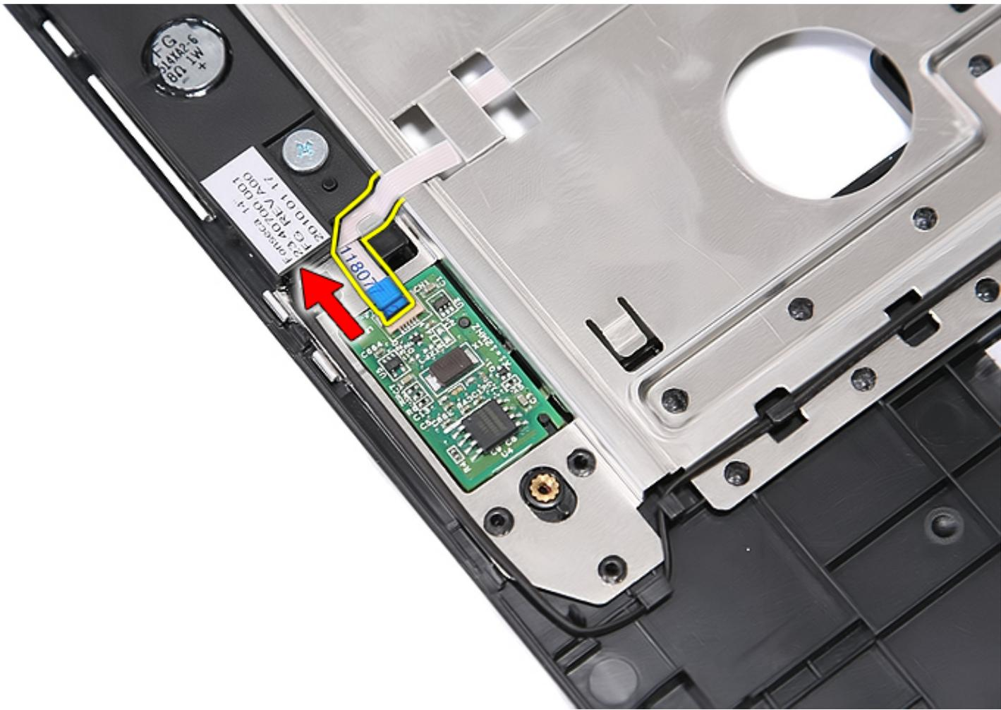
14. Lift up the fingerprint reader board and remove it.
