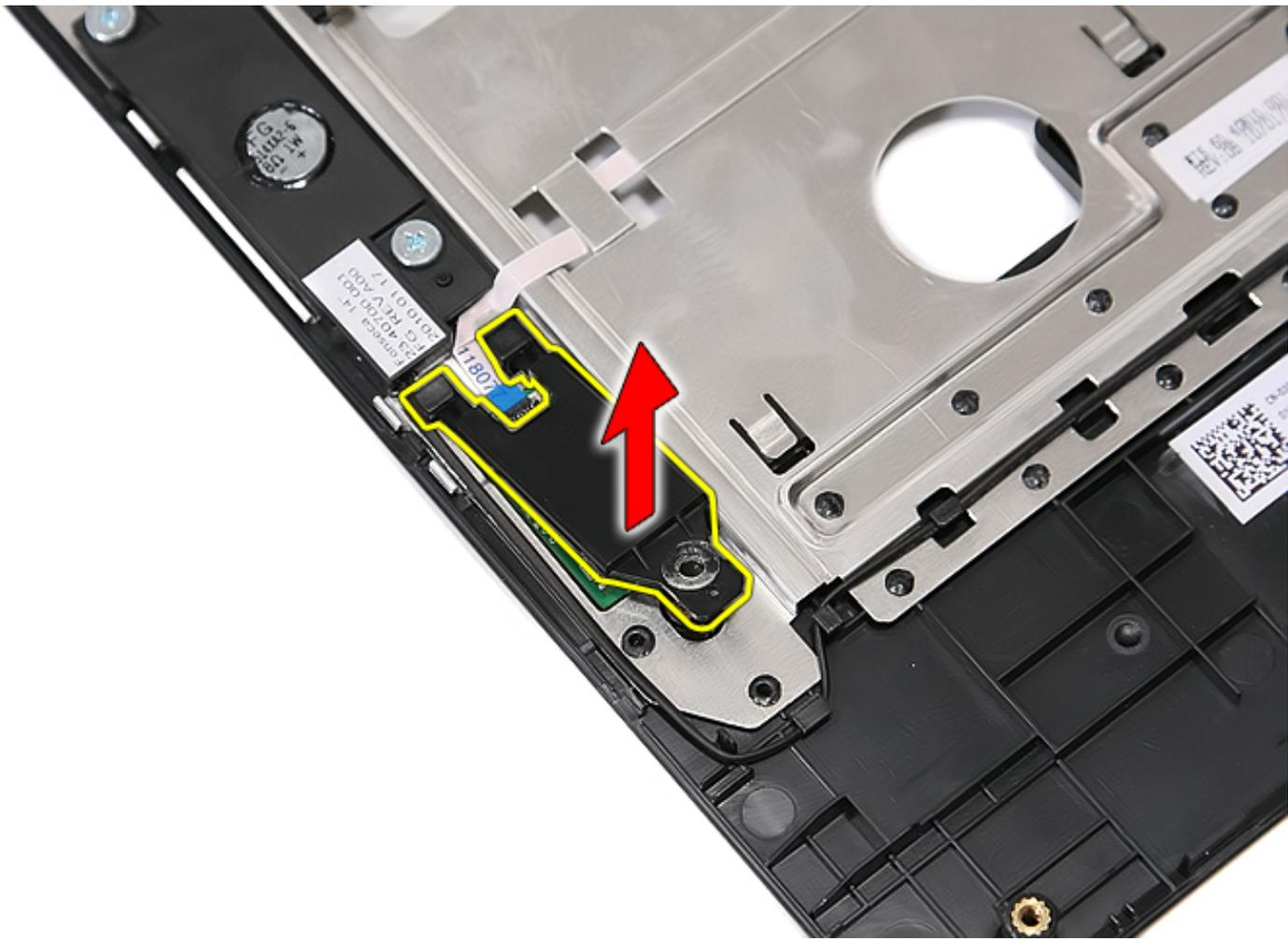
12. Open the fingerprint reader data cable-securing clip.
