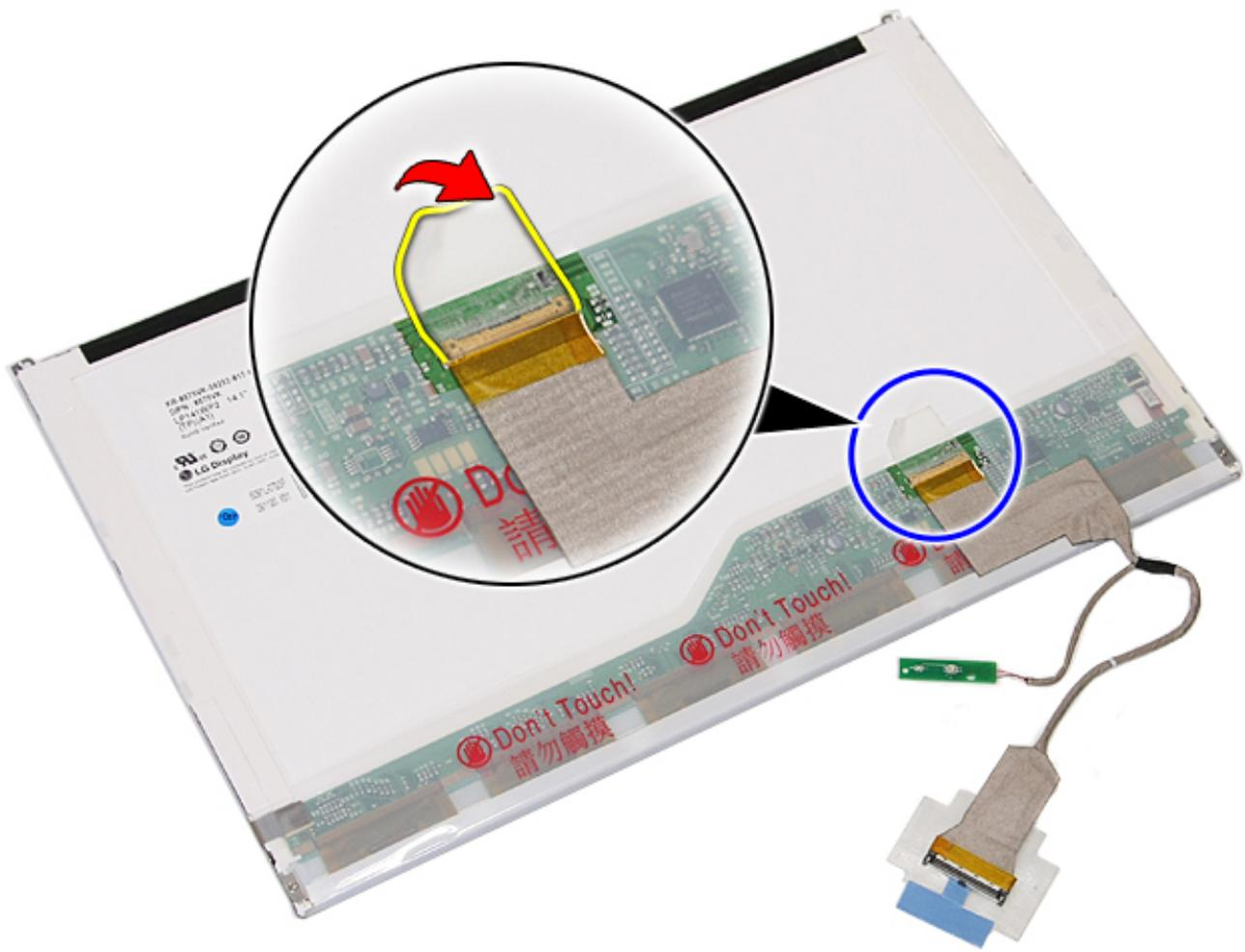
14. Disconnect the display cable from the display panel.
