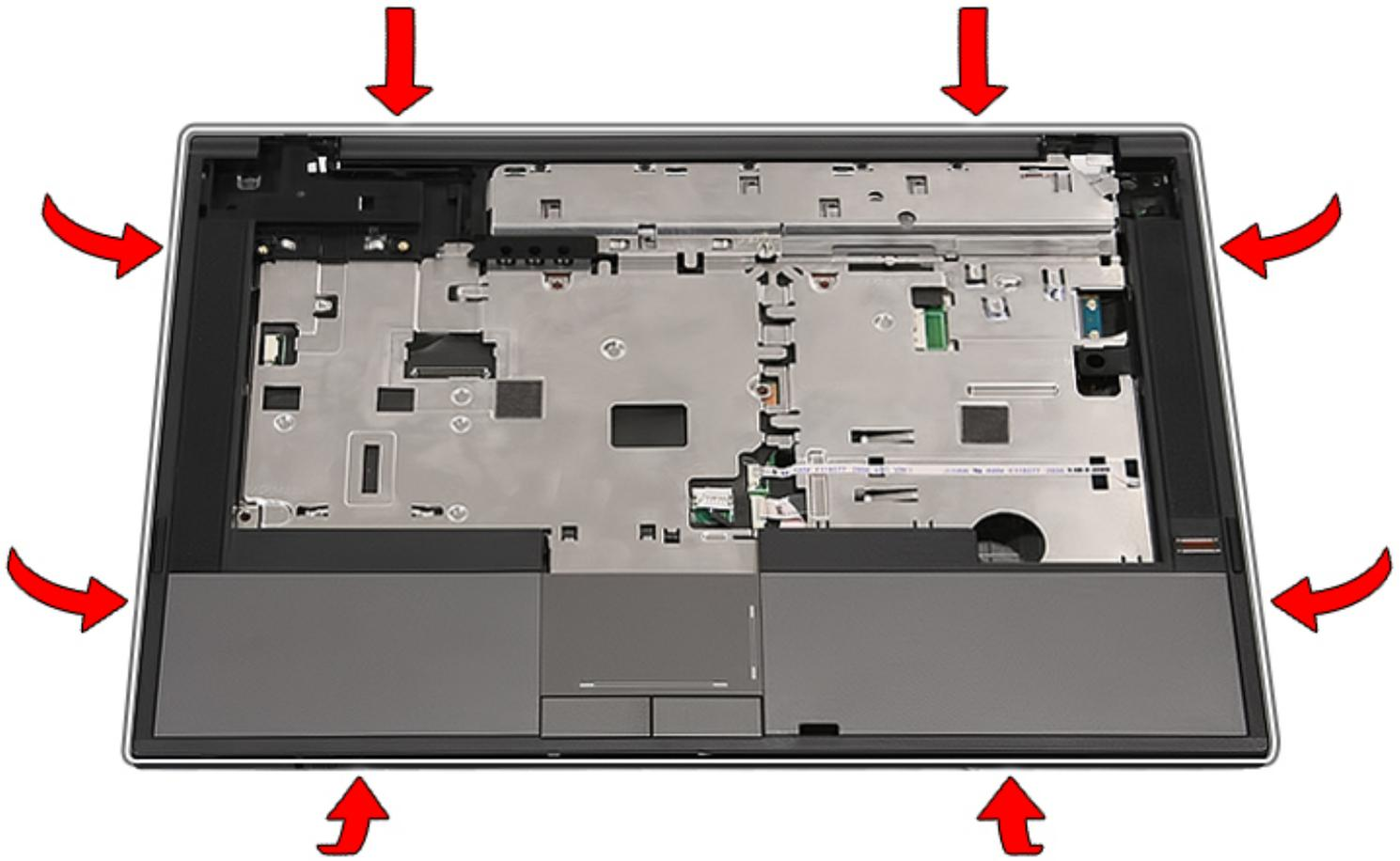
20. Lift up the palm rest from the computer and remove it.
