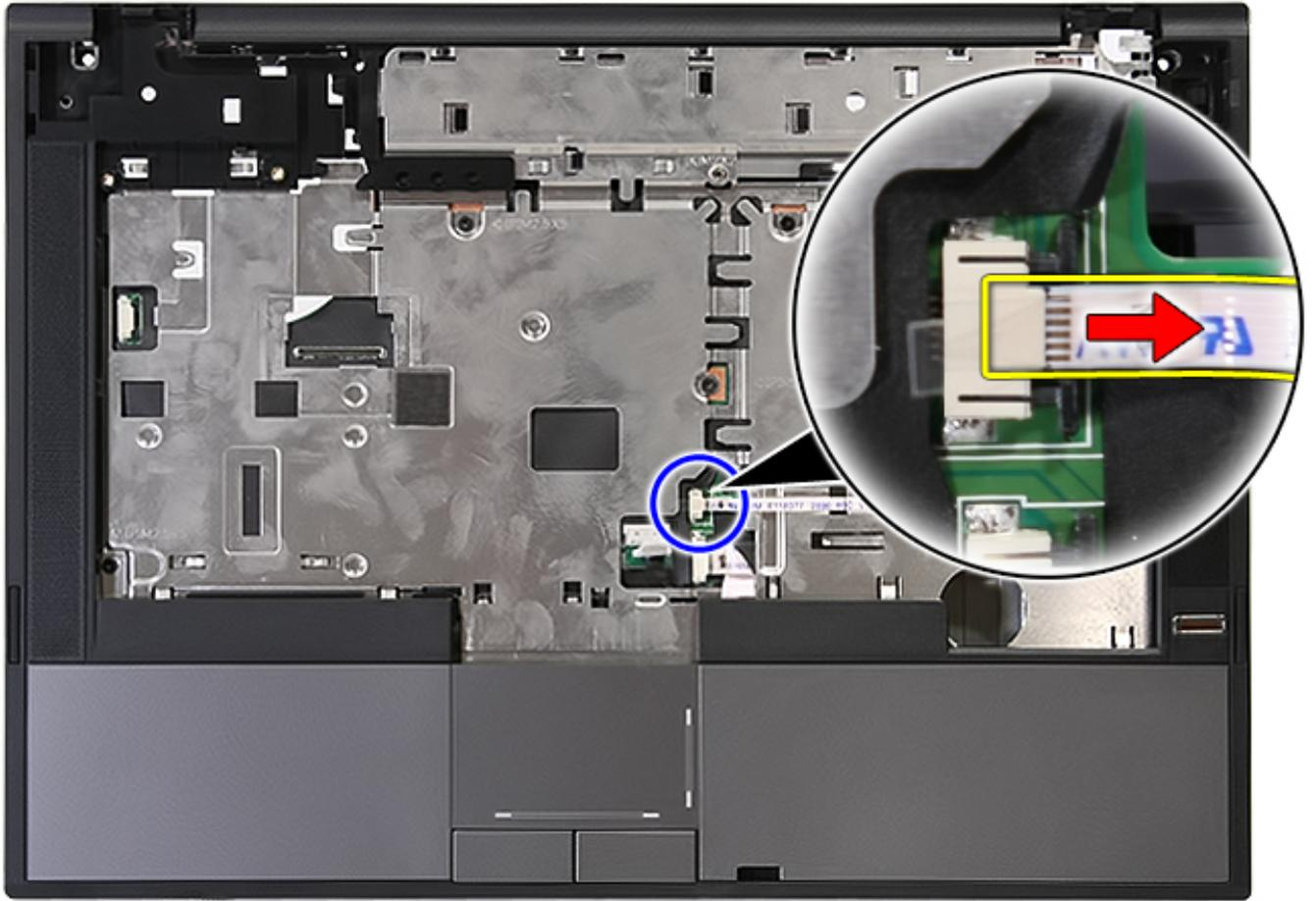
16. Release the latch securing the touchpad data cable.
