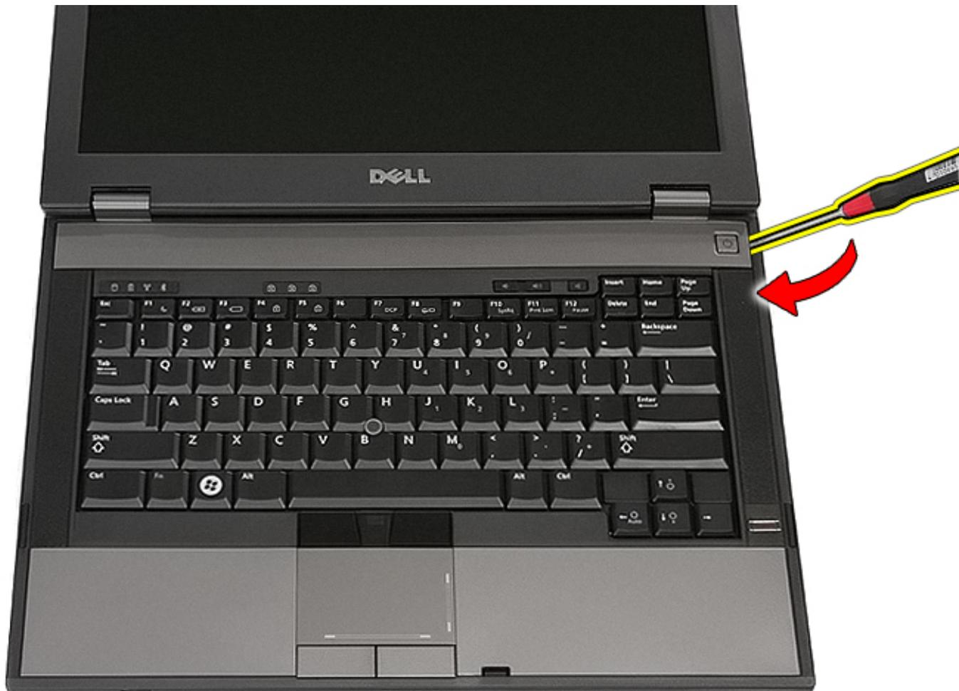
4. Gently pry along the edge of the LED cover to release it from the latches and remove.
