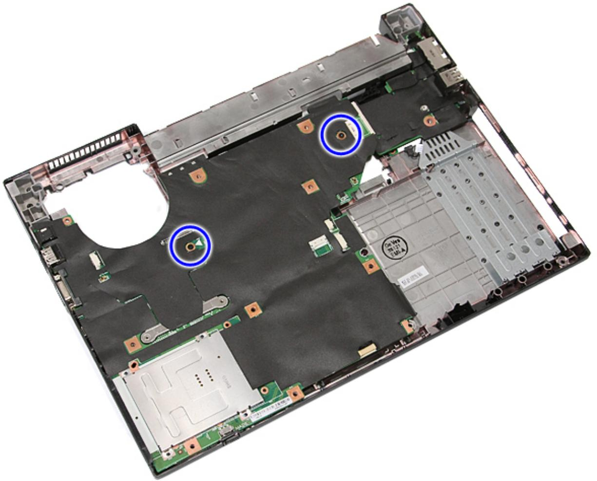
19. Lift the system board at an angle and remove it.
