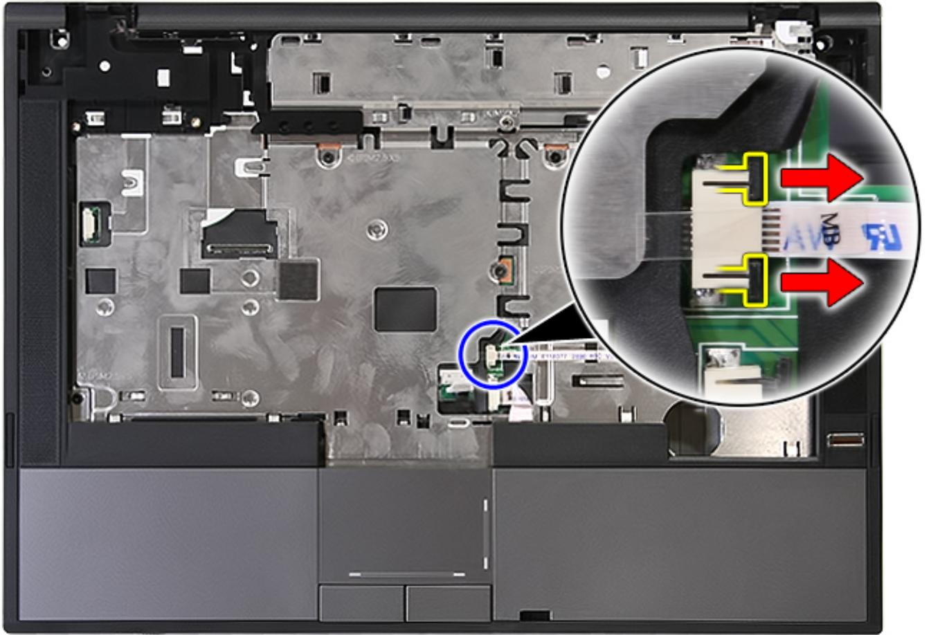
15. Disconnect the fingerprint reader data cable.
