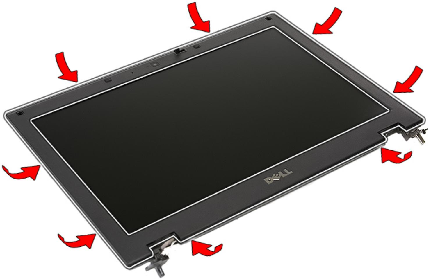
11. Lift up and remove the display bezel from the computer.
