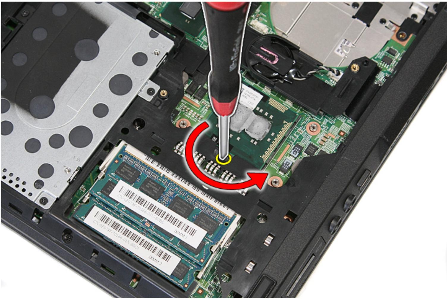
7. Lifting straight up, remove the processor from the computer.
