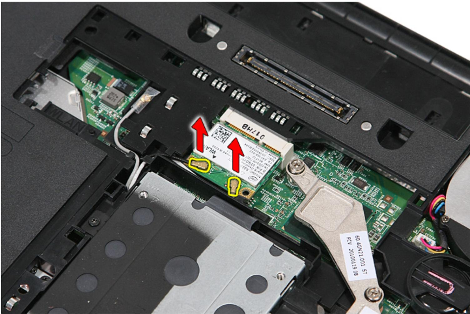
5. Gently pry the latch to release the WLAN card.
