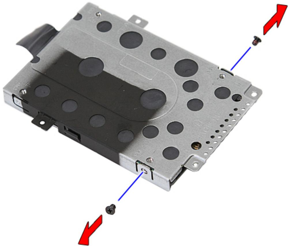
7. Lift up the hard drive caddy at an angle from the hard drive and remove.
