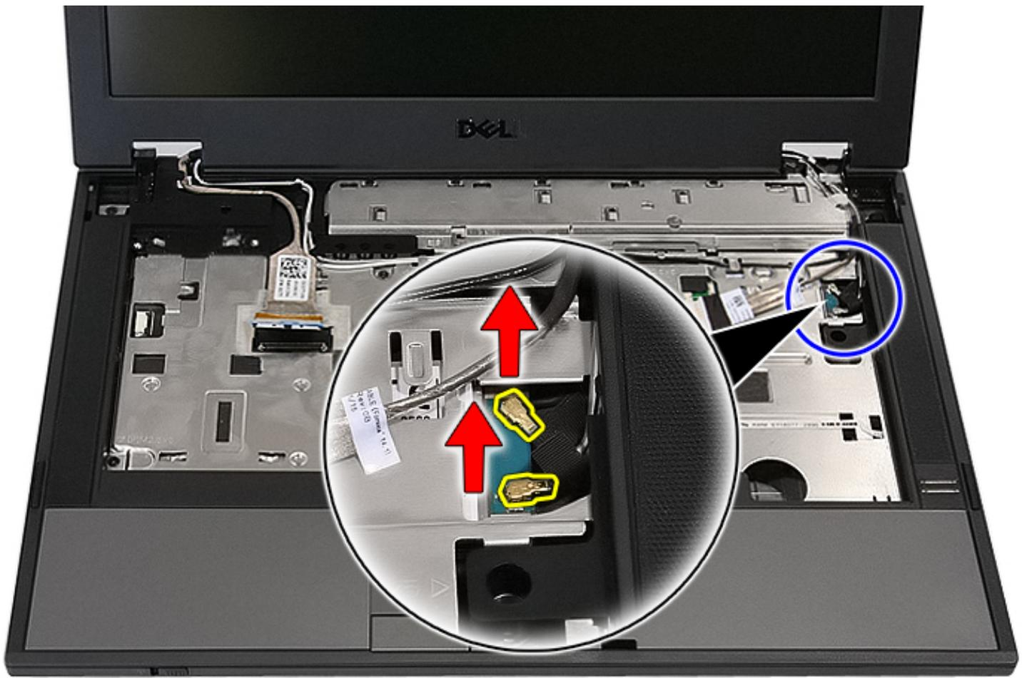
12. Release the cables from the routing path.
