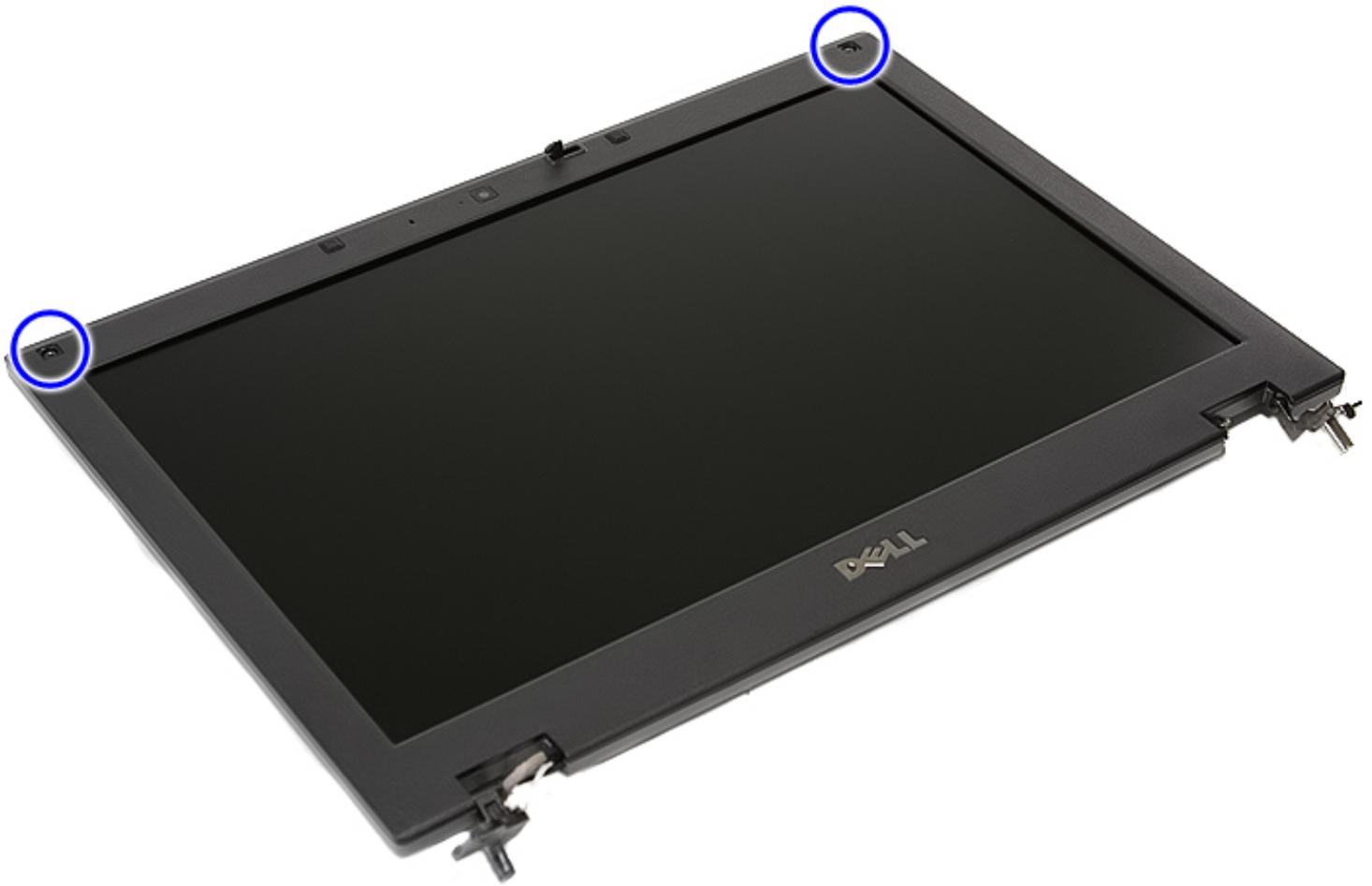
10. Gently pry the display bezel from the display assembly by tucking your fingers under one edge of the bezel and working your way around the entire bezel until it is completely free.
