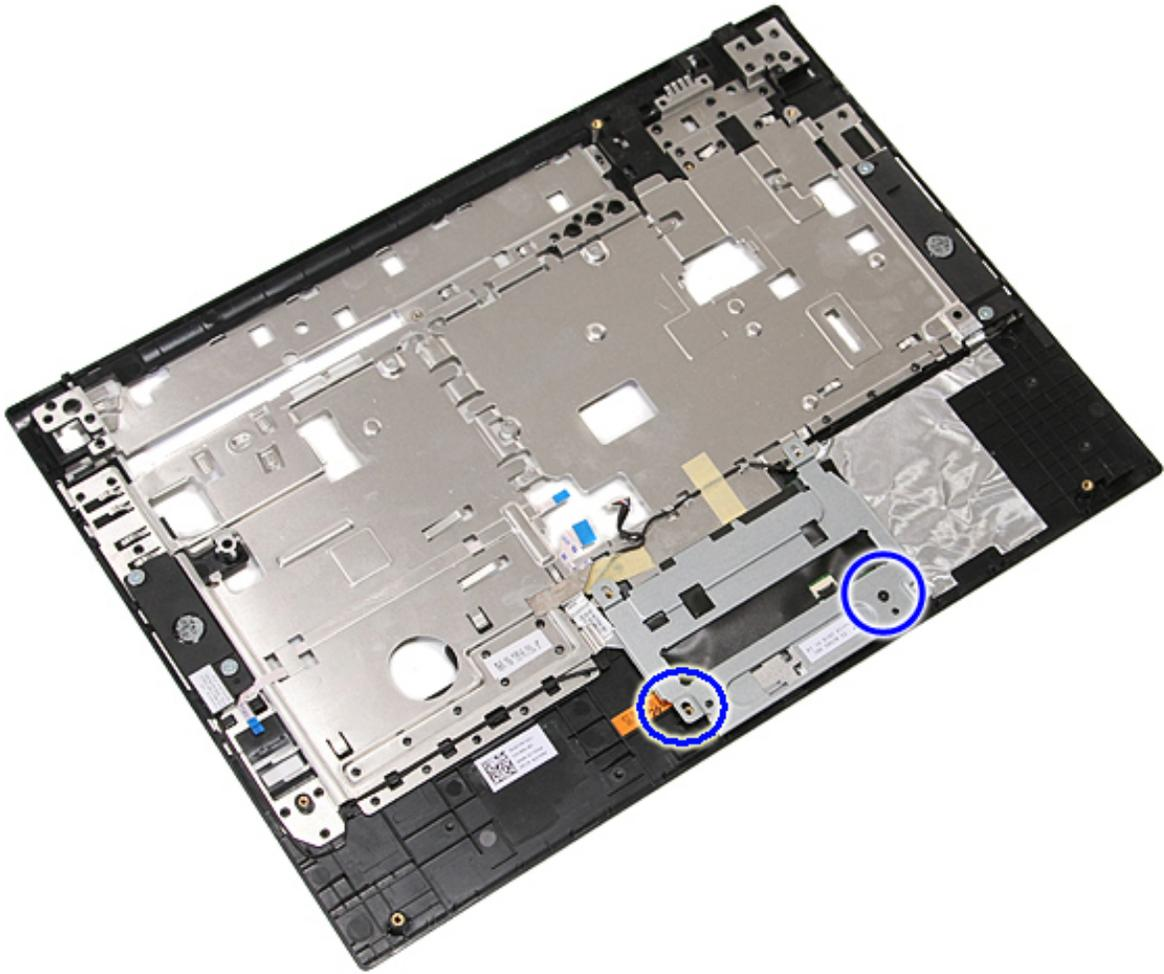
12. Lift up the touchpad cover bracket and remove it.
