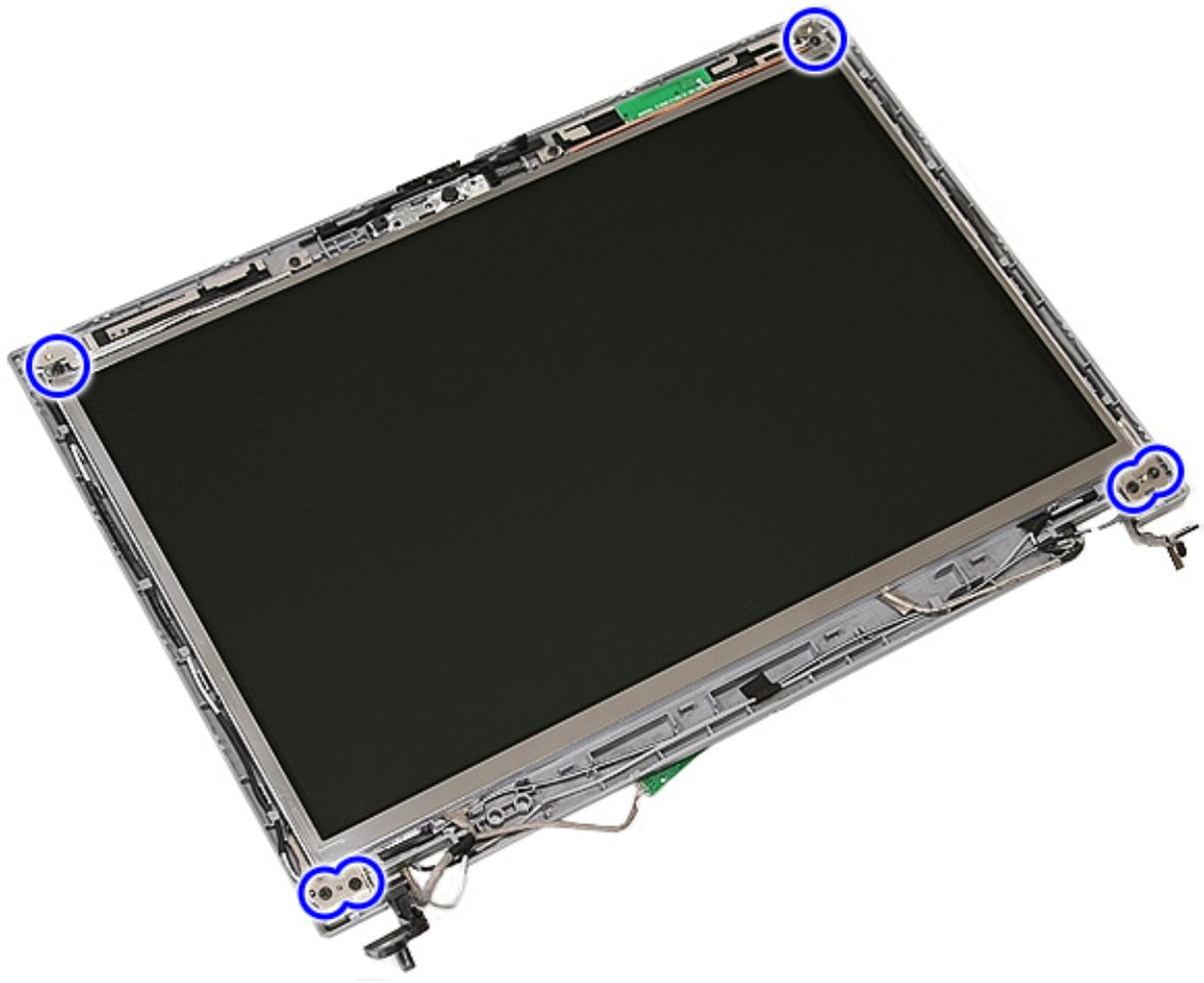
11. Lift up the display panel, brackets, and hinges.
