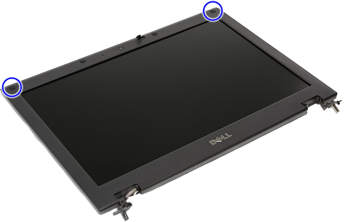
9. Remove the screws securing the display bezel to the display cover.
