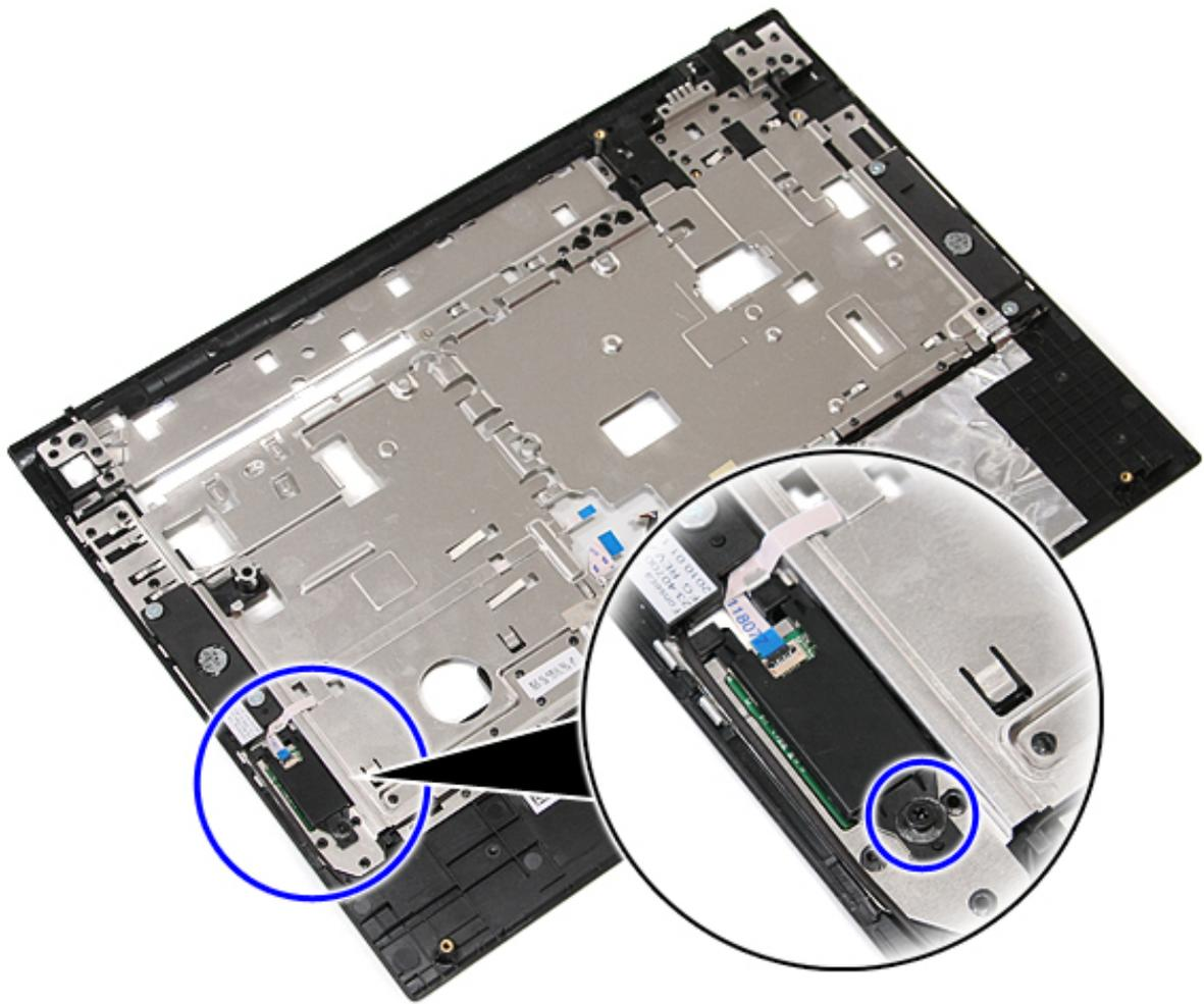
11. Lift up the fingerprint reader cover at an angle and remove.
