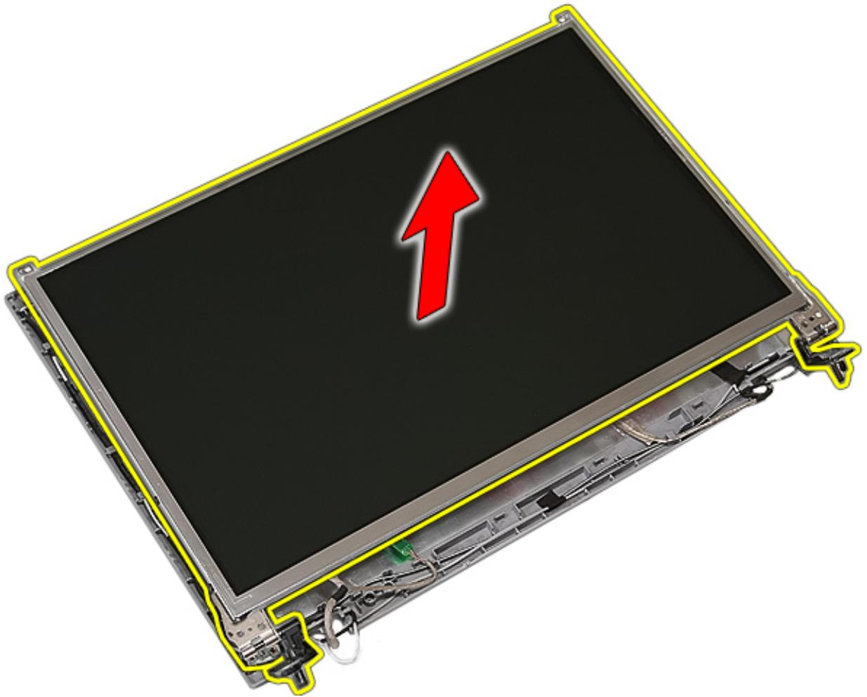
12. Remove the screws securing the display brackets and hinges to the display panel and remove.
