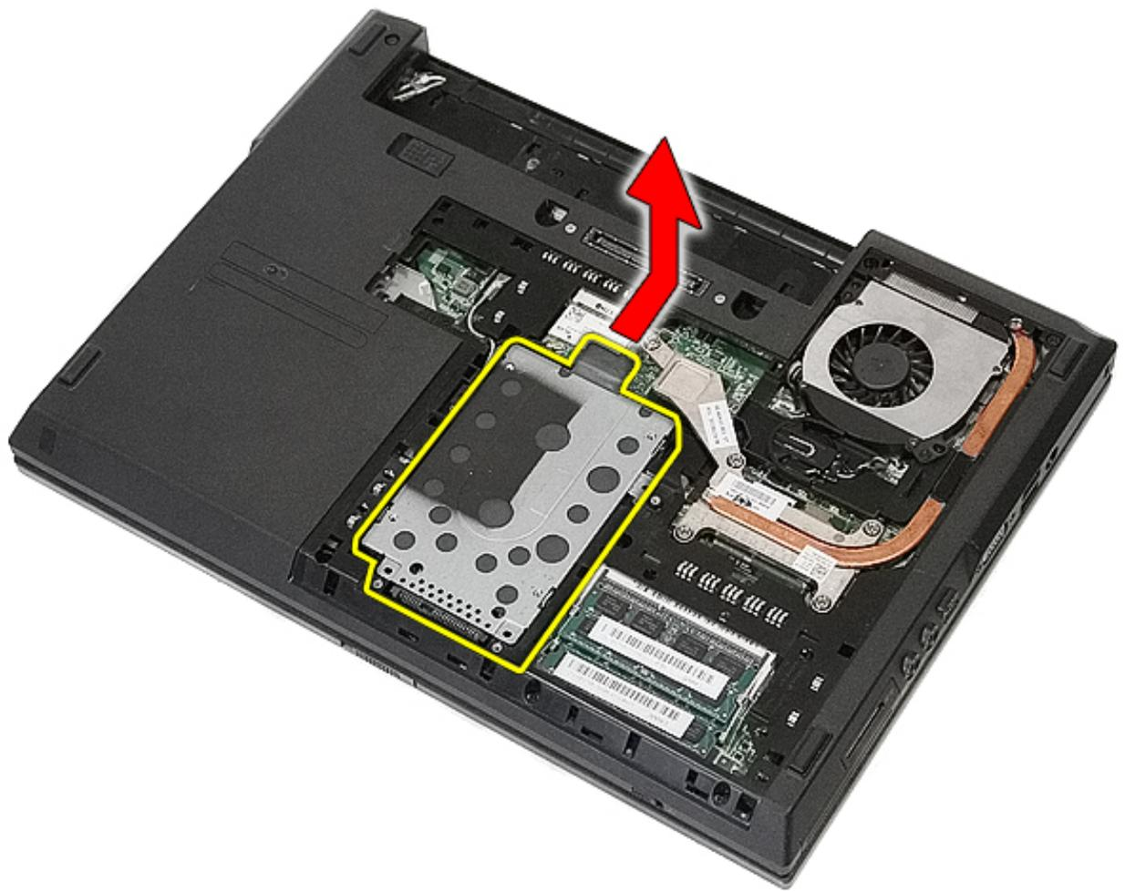
6. Remove the screws securing the hard drive caddy to the hard drive.
