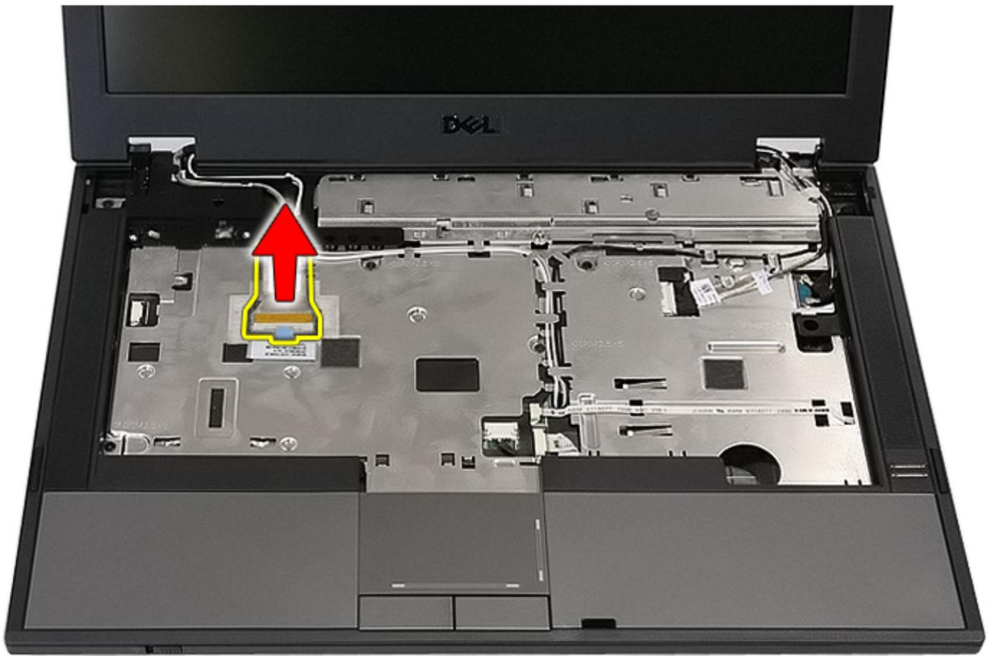
10. Disconnect the camera cable from the system board.
