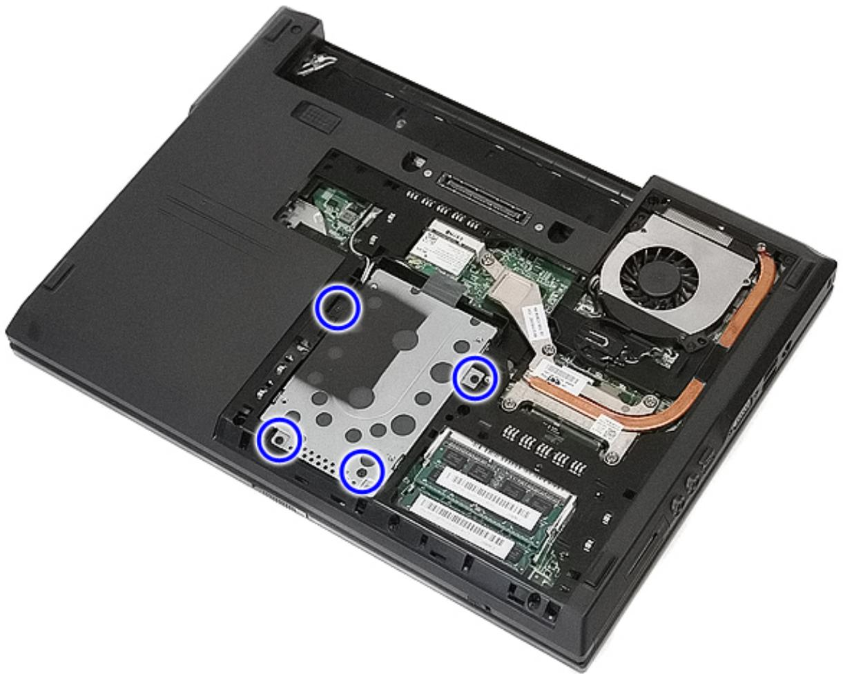
5. Slide the hard drive towards the center of the computer and remove.
