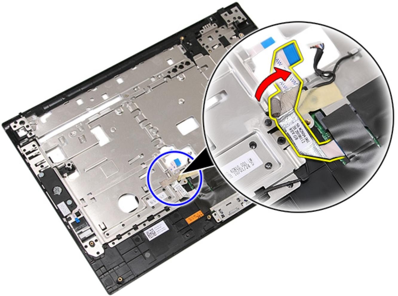
15. Release the speaker cables from the routing path.
