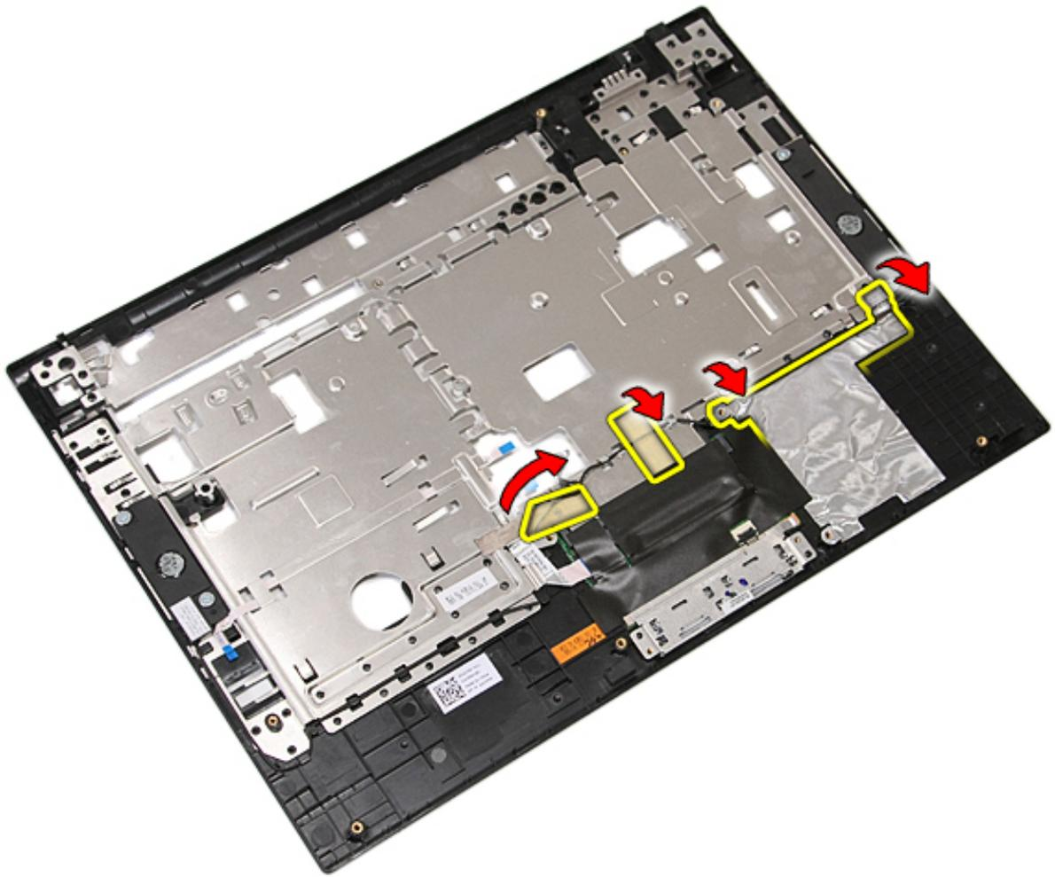
14. Peel open the tape securing the touchpad data cable to the palm rest, and pull out the cable from the hole.
