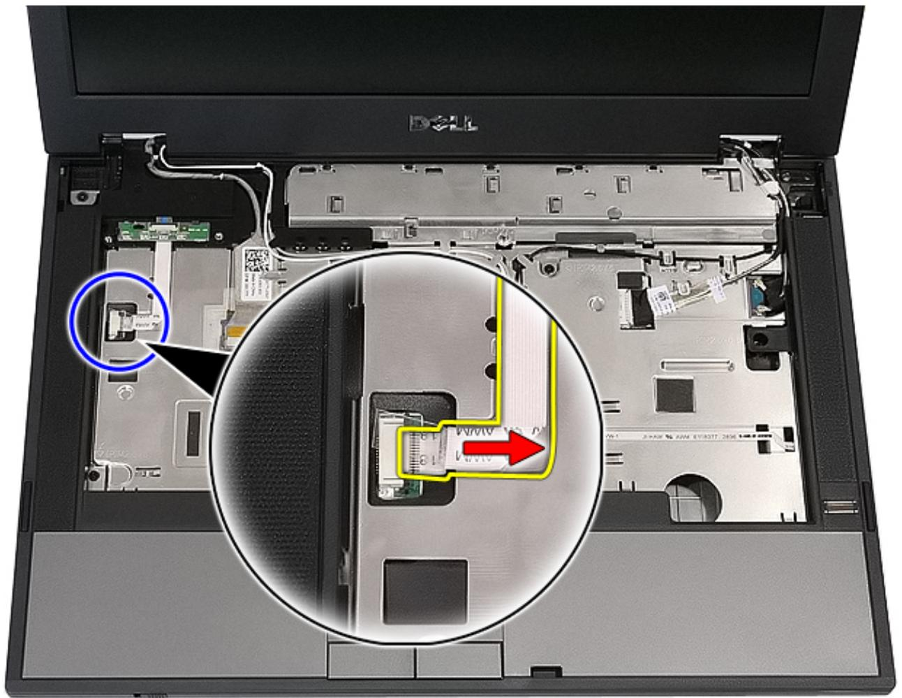
7. Release the latches securing the LED Board and remove.
