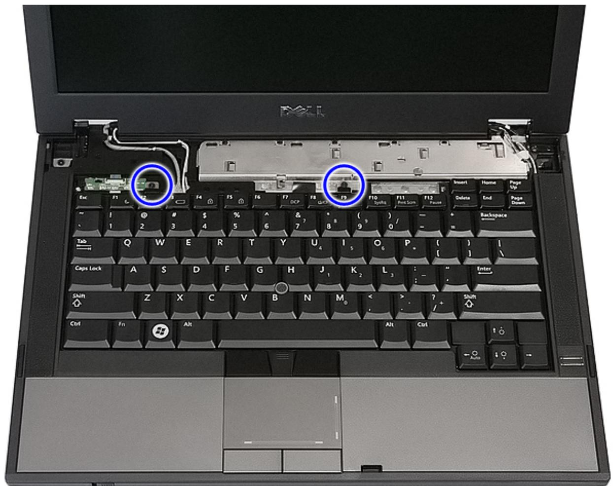
5. Slide the keyboard upwards, then lift and remove the keyboard from the computer.
