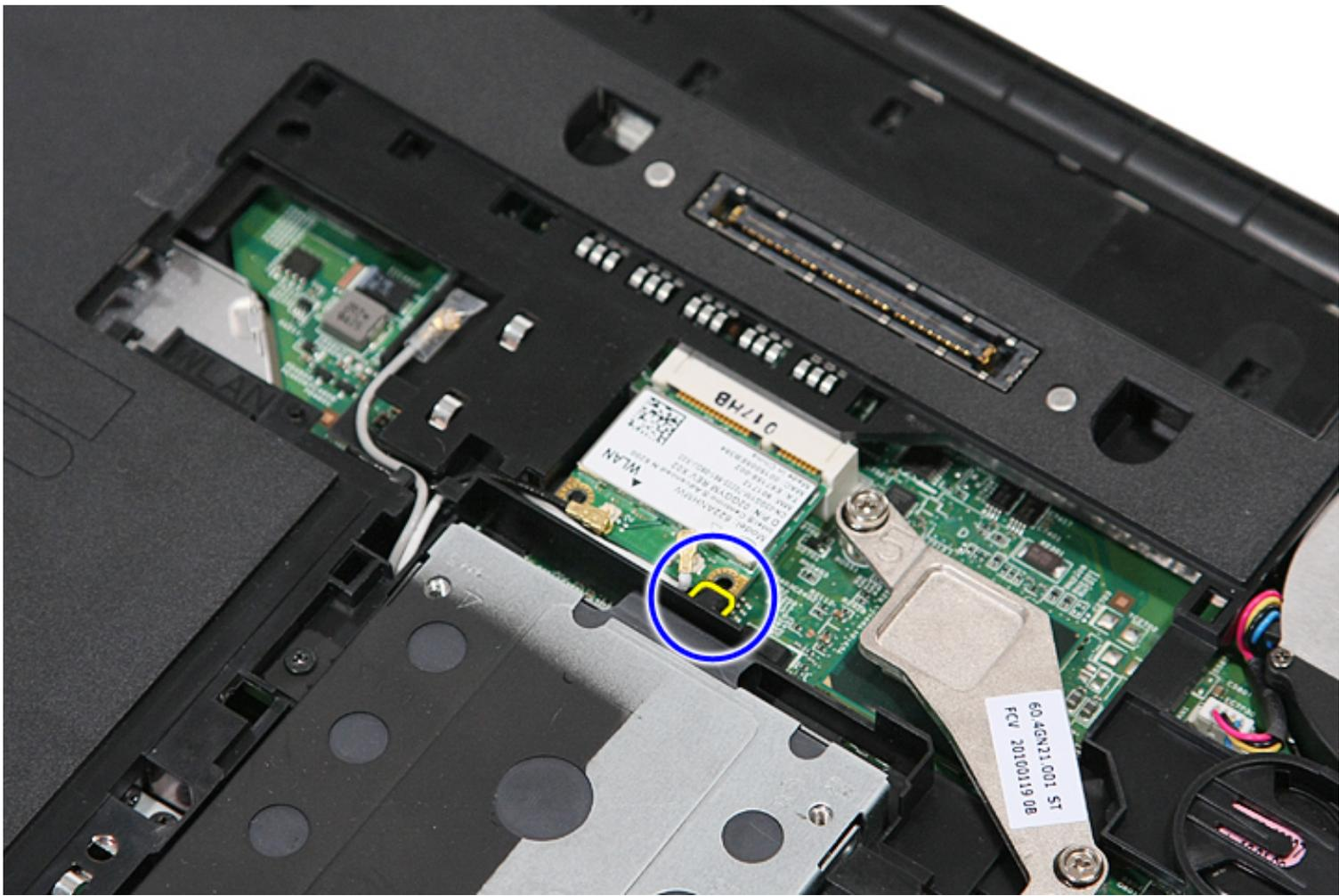
6. Remove the WLAN card from the computer.
