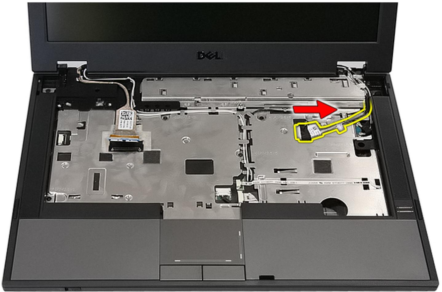
11. Release the antenna cables from the WWAN card (if installed).
