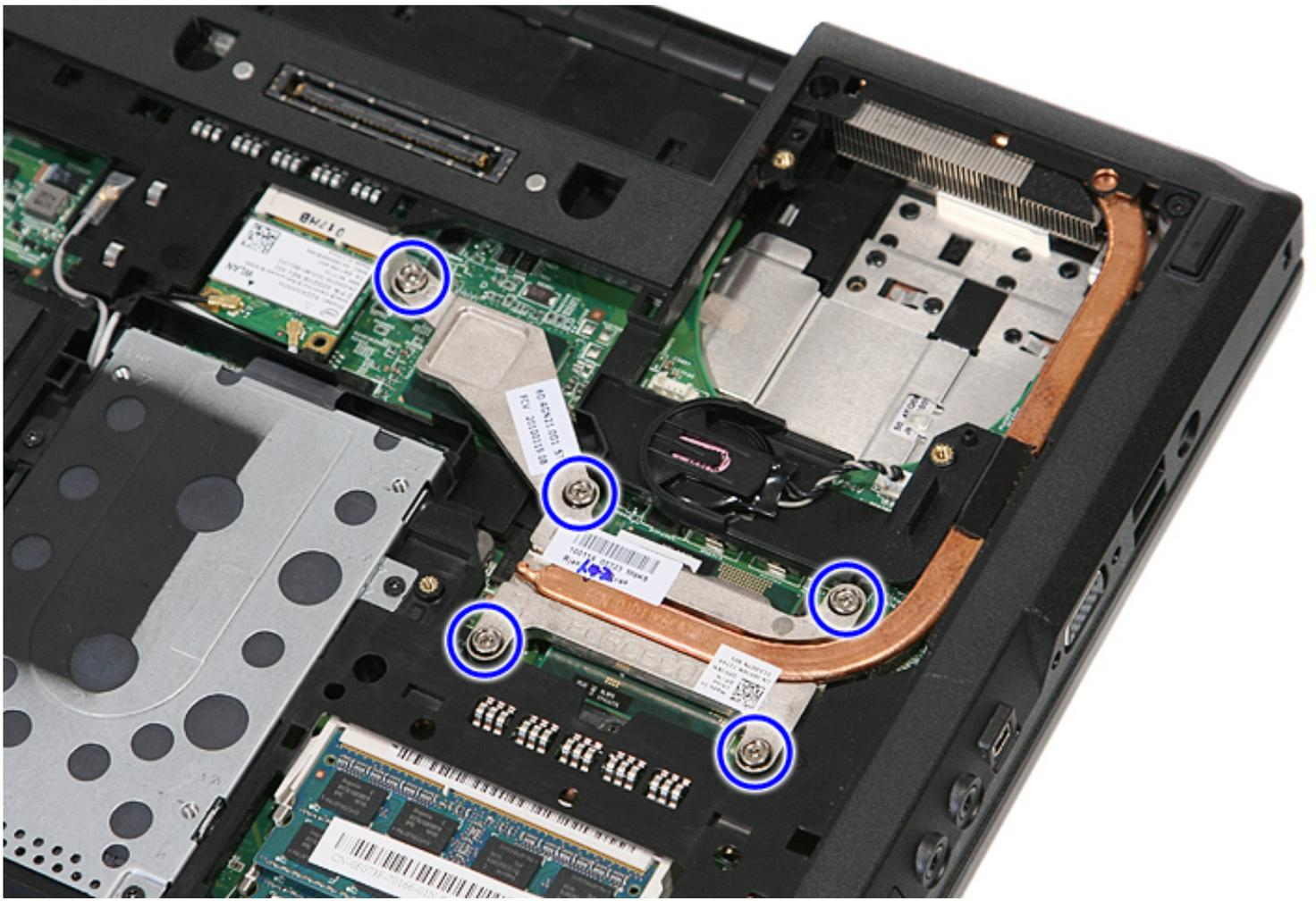
6. Lift up the heat sink at an angle and remove it from the computer.
