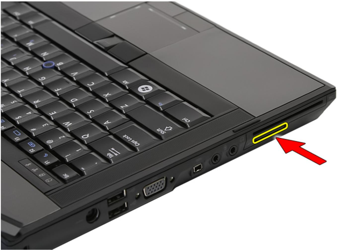
4. Slide the memory card out of the computer and remove.
