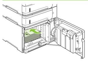
**5.** Make sure that the height of the stack does not exceed the maximum-height indicators on the guides and that the front edge of the stack is aligned with the arrows.
