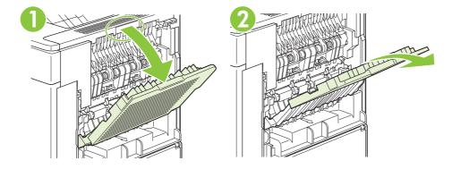
Opening the rear output bin makes the duplexer (if installed) and the top output bin unavailable. To avoid jams, do not open or close the rear output bin while the product is printing.
