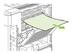
NOTE: If the jammed paper is difficult to remove, try opening the top cover all the way to release pressure on the paper. If the sheet has torn, or if you still cannot remove it, see <u>Clear jams from the fuser area on page 170</u>.
