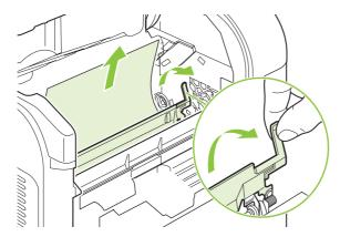
3. Open Tray 1 and remove the envelope accessory cover. If paper is present, remove it.
