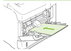
4. Adjust the side guides so that they lightly touch the paper stack but do not bend the paper.
