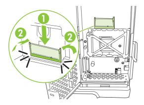
MOTE: To remove a DIMM, first release the locks.
