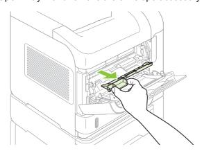
**4.** Rotate the paper guide to check for additional jammed paper underneath. If jammed paper is present, remove it.
