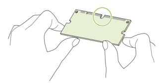
Press the DIMM straight into the slot, and press firmly. Make sure the locks on each side of the DIMM snap into place.
