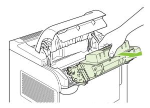
3. Remove the new print cartridge from the bag. Place the used print cartridge in the bag for recycling.
