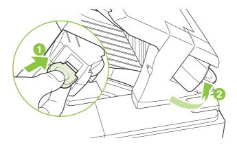
The stapler needs to reload after clearing a staple jam, so the first few documents might not be stapled. If a print job is sent and the stapler is jammed or is out of staples, the job will still print as long as the path to the stacker bin is not blocked.
