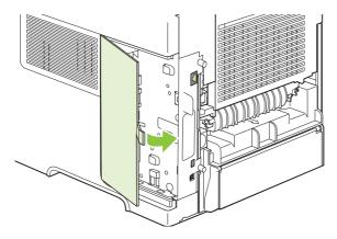
9. Reinstall the right-side panel. Align the tabs on the panel with the slots in the product, and push the panel toward the front of the product until it latches into place.
