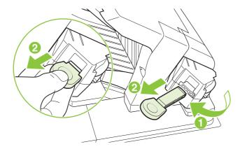
Insert the new staple cartridge into the stapler unit and rotate the stapler unit toward the rear of the product until the unit snaps into place.
