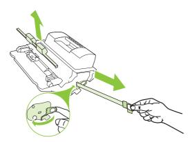
Align the print cartridge with the tracks inside the product, insert the print cartridge until it is firmly seated, and then close the top cover.
