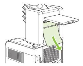
4. If the paper is jammed at the bottom of the 5-bin mailbox, open the rear output bin, and then pull straight up on the paper to remove it.
