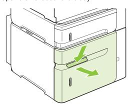
2. If the edge of the jammed paper is visible in the feed area, slowly pull the paper down and out of the product. (Do not pull the paper straight out, or it will tear.) If the paper is not visible, look in the top-cover area. See <u>Clear jams from the top-cover and print-cartridge areas on page 162</u>.
