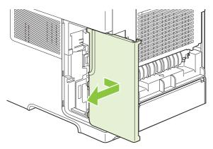
Open the access door by pulling on the metal tab.
