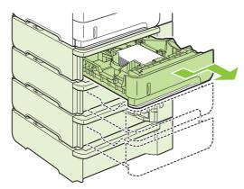
Pinch the release that is located on the left guide and slide the side guides to the correct paper size.
