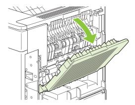
4. Remove the rear output bin. Place your finger near the left-side hinge, and push firmly to the right until the hinge-pin clears the hole inside the product. Rotate the output bin outward to remove it.
