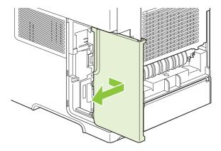
4. Open the access door by pulling on the metal tab.
