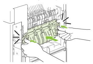
**8.** Reinstall the rear output bin. Insert the right hinge-pin into the hole inside the product. Push inward on the left hinge, and slide it into the hole inside the product. Close the rear output bin.
