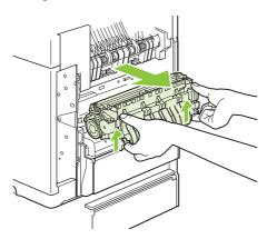
6. Remove the jammed paper. If necessary, lift the black plastic guide that is located on the top of the fuser to gain access to the jammed sheet.
