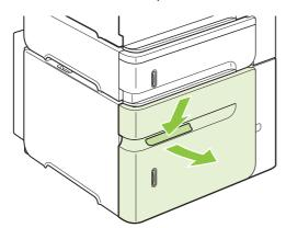
2. If paper is in the tray, remove it. When paper is in the tray, the guides cannot be adjusted.
