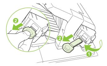
2. Rotate the green cover on the end of the staple cartridge upward, and remove the jammed staple.
