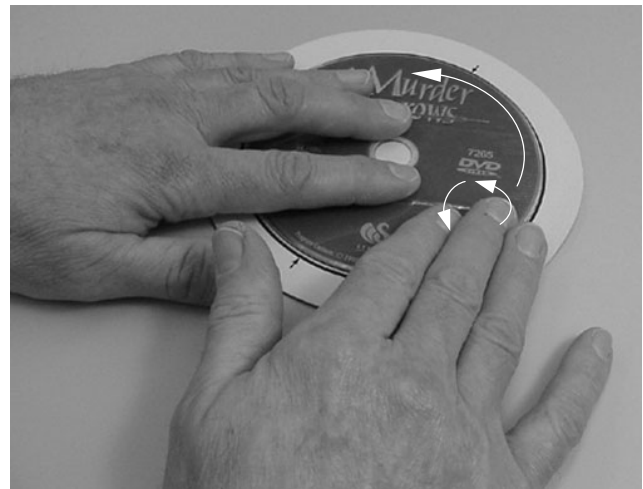
Figure 5: Adhering overlay to entire disc surface.
