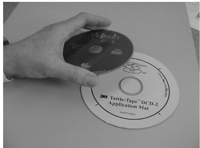
Figure 1: Placing disc within alignment circle on application mat.
