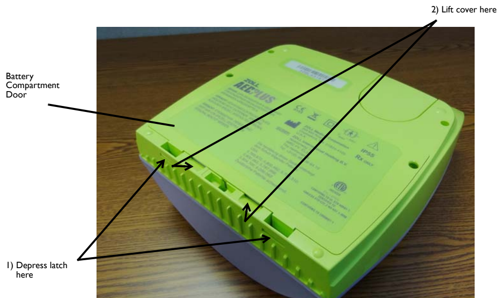
Figure 7: Removing the Battery Compartment Door
