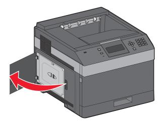
Loosen the screws on the system board cover.
