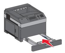
**8** If a different type of paper was loaded than the type previously loaded in the tray, then change the Paper Type setting for the tray from the printer control panel.
