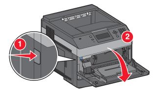
2 Press the button on the base of the photoconductor kit, and then pull the toner cartridge out using the handle.
